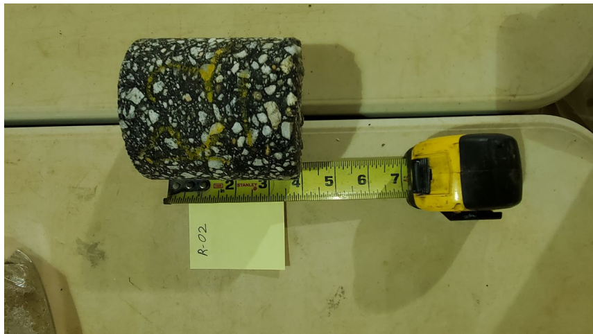
Photo 8: Core at R-02 (Core oriented with asphalt surface to the left)
