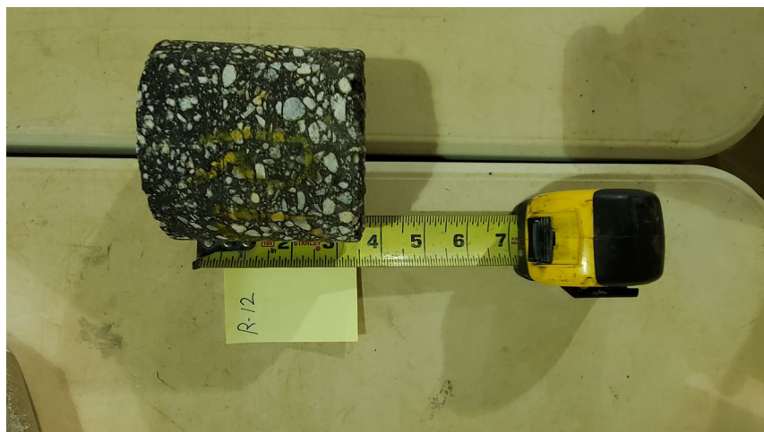
Photo 18: Core at R-12 (Core oriented with asphalt surface to the left)
