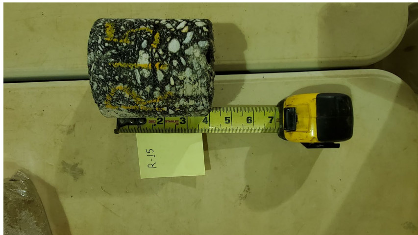
Photo 21: Core at R-15 (Core oriented with asphalt surface to the left)
