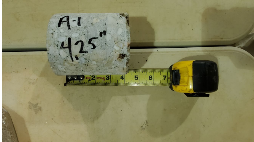
Photo 1: Core at A-01 (Core oriented with concrete surface to the left)
