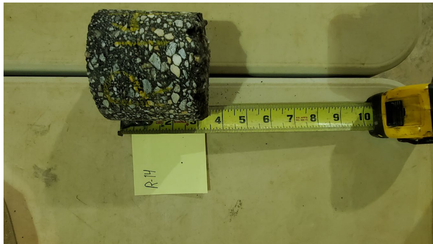
Photo 20: Core at R-14 (Core oriented with asphalt surface to the left)
