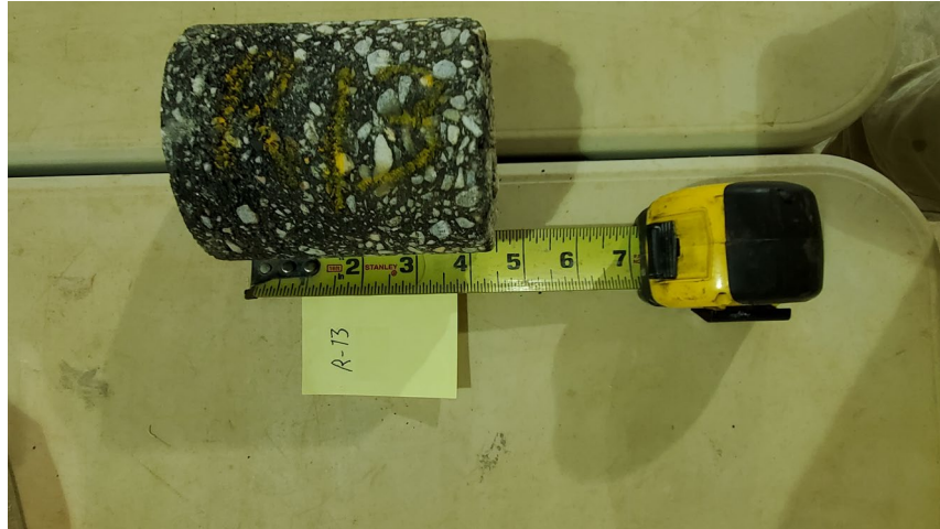
Photo 19: Core at R-13 (Core oriented with asphalt surface to the left)
