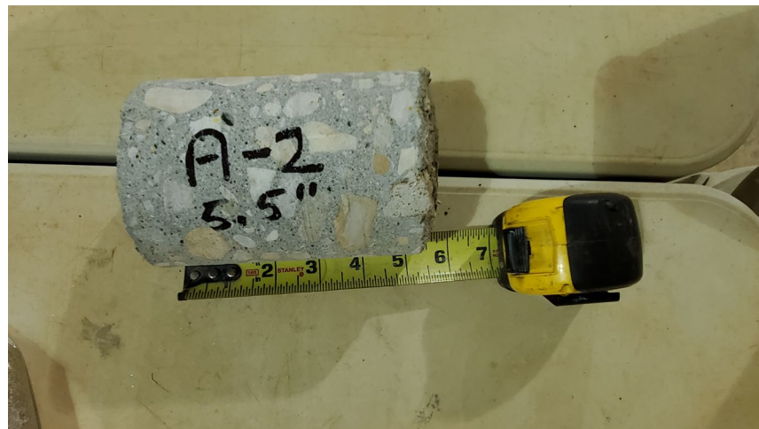
Photo 2: Core at A-02 (Core oriented with concrete surface to the left)
