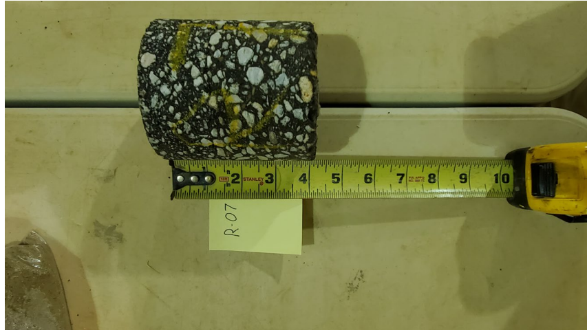
Photo 13: Core at R-07 (Core oriented with asphalt surface to the left)
