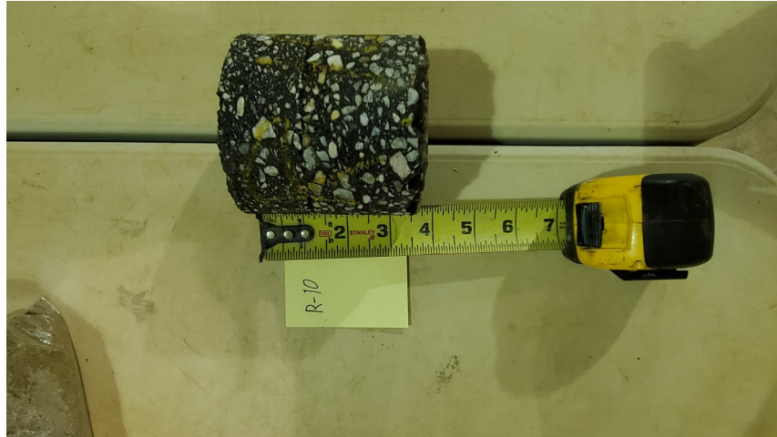
Photo 16: Core at R-10 (Core oriented with asphalt surface to the left)
