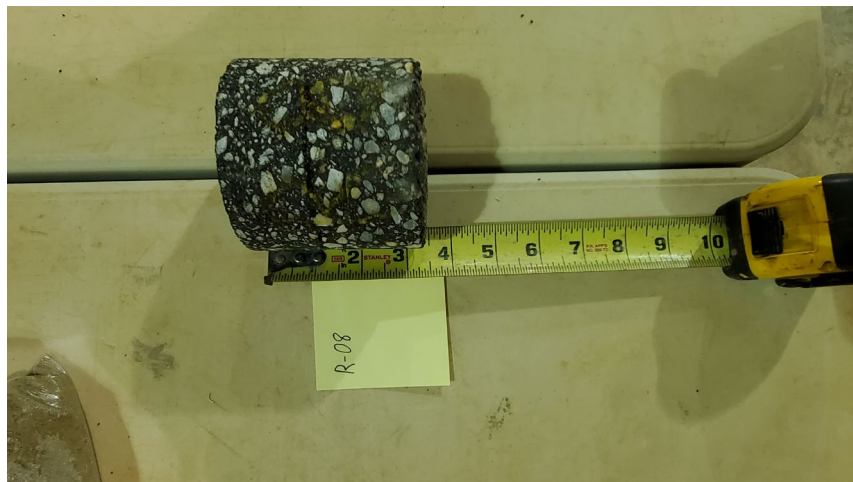
Photo 14: Core at R-08 (Core oriented with asphalt surface to the left)
