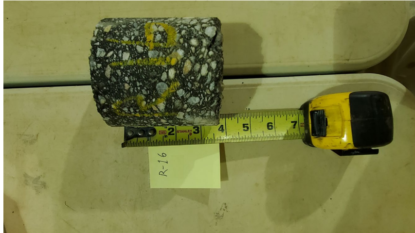
Photo 22: Core at R-16 (Core oriented with asphalt surface to the left)
