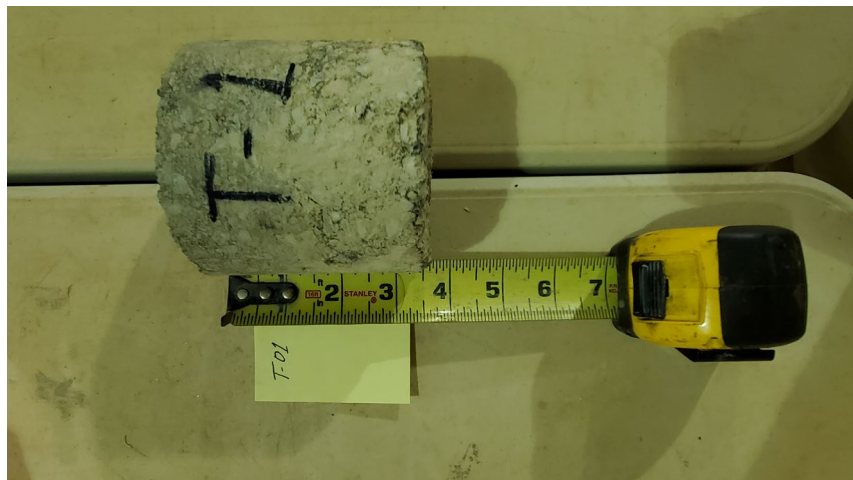
Photo 24: Core at T-01 (Core oriented with asphalt surface to the left)
