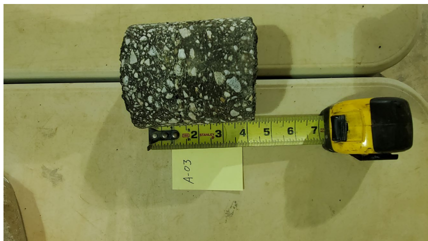
Photo 3: Core at A-03 (Core oriented with asphalt surface to the left)
