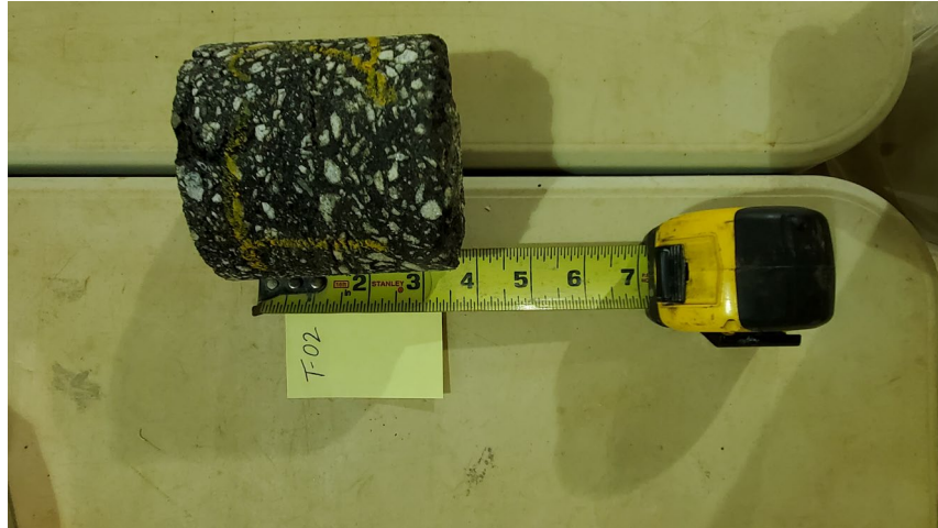
Photo 25: Core at T-02 (Core oriented with asphalt surface to the left)
