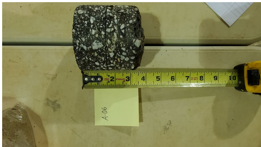
Photo 6: Core at A-06 (Core oriented with asphalt surface to the left)
