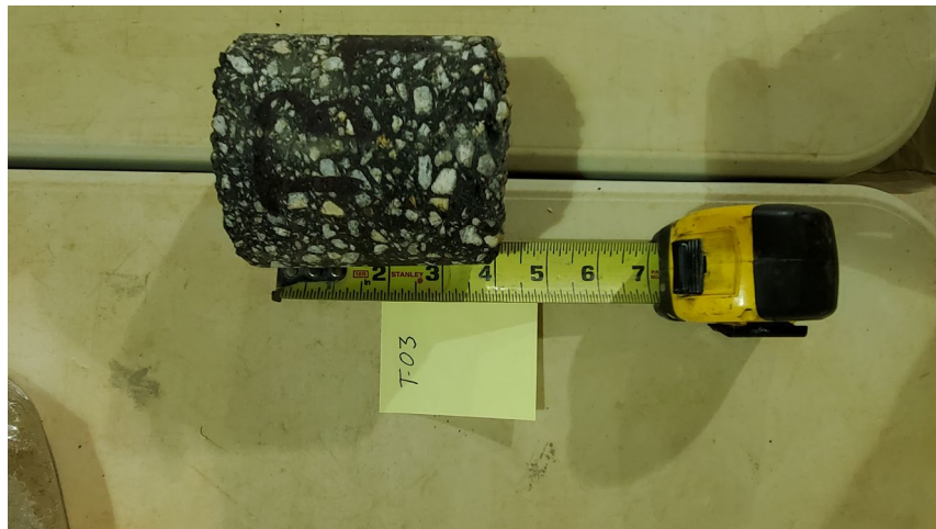
Photo 26: Core at T-03 (Core oriented with asphalt surface to the left)
