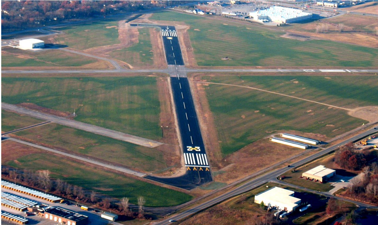
Figure 2-3. Markings for a Temporarily Closed Runway
