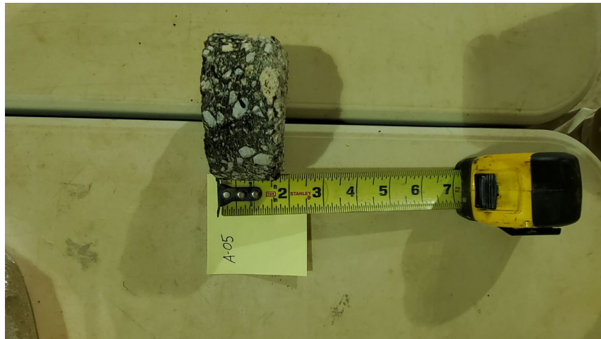
Photo 5: Core at A-05 (Core oriented with asphalt surface to the left)
