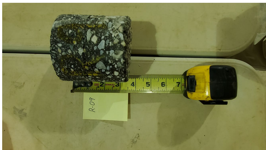
Photo 15: Core at R-09 (Core oriented with asphalt surface to the left)
