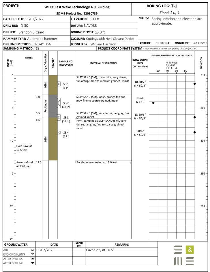
GROUNDWATER DEPTHS ARE NOT EXACT AND MAY VARY SUBSTANTIALLY FROM THOSE INDICATED. ATD = AT TIME OF D RILLING LL=Liquid Limit, PL = Plastic Limit, NMC = Natural Moisture Content, PPV = Pocket Penetrometer (tsf), PTV = Pocket Torvane (tsf), AR = Auger Refusal
