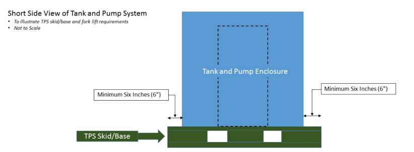
Fork Lift pockets must be placed so that when a fork lift is used the TPS is balanced
